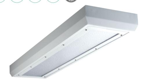
IP54 and IK10 vandal resistant luminaires. Constructed from a rigid steel body and 6mm thick cracked ice polycarbonate diffuser, secured by tamper-proof stainless steel bolts. Suitable for use in secure installations, as well as public areas such as subways, bus stations and other vandal prone areas. IK10 rated, vandal resistant construction
